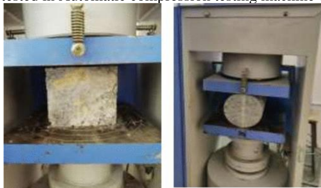
Figure 4. Compressive strength test and Split tensile test of PUMICE lightweight aggregate concrete cube and cylindrical specimen respectively with Automatic compression testing machine of 2000kN capacity
