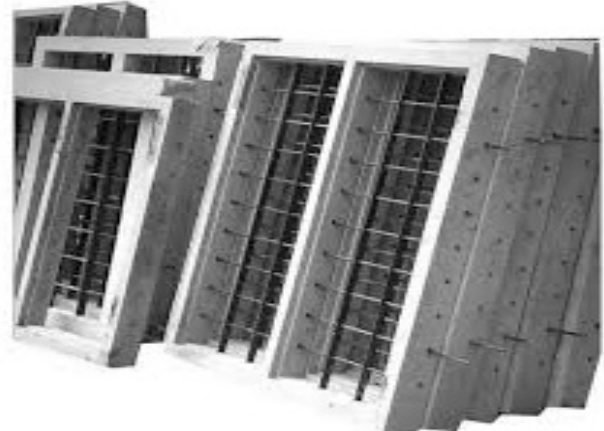
Fig. 6: RCC Window Frames
