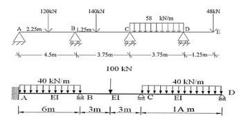
11. Analyse and design the RCC beam for the following support and load conditions. Show SFD and BMD.
